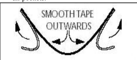
◀ Fig 6. Ultraseal Tape: centralise over area to be protected and press down firmly to form a bond, removing interleaving as you progress.
