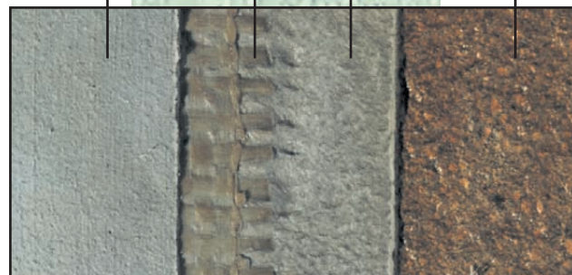
700 Series showing stages of coating
