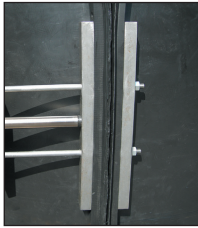
2. This allows the seams to be bolted under improved stretch and tension.
