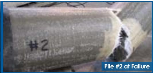
Pile #2 at Failure
