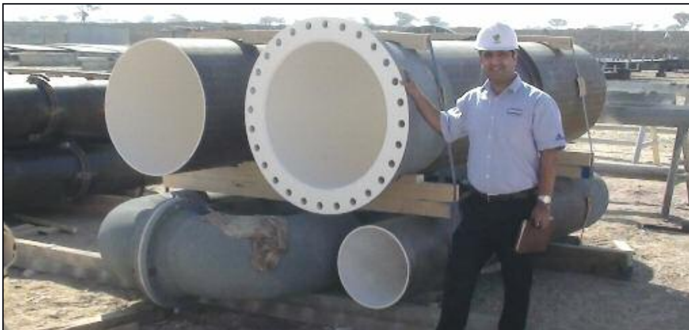
Sea water intake pipes lined with Archco-Rigidon Rigspray
