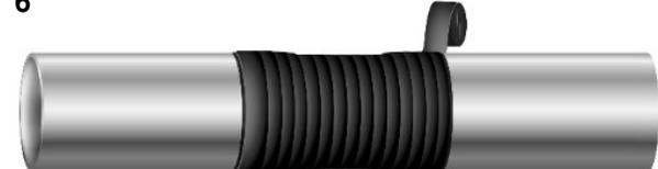
Wrap a second layer of Denso S43 HT Tape with a 55% overlap using slight tension and without folds. The grey compound is to be in contact with the black outer layer of the previous wrap. The outer wrap must cover the inner wrap at the edges with minimum 25 mm, so that now minimum 75 mm of the factory coating, painted initially in a width of approx. 100 mm, are incorporated into the site applied coating.
