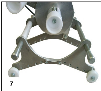
7 Wheel position for \geq DN 600
