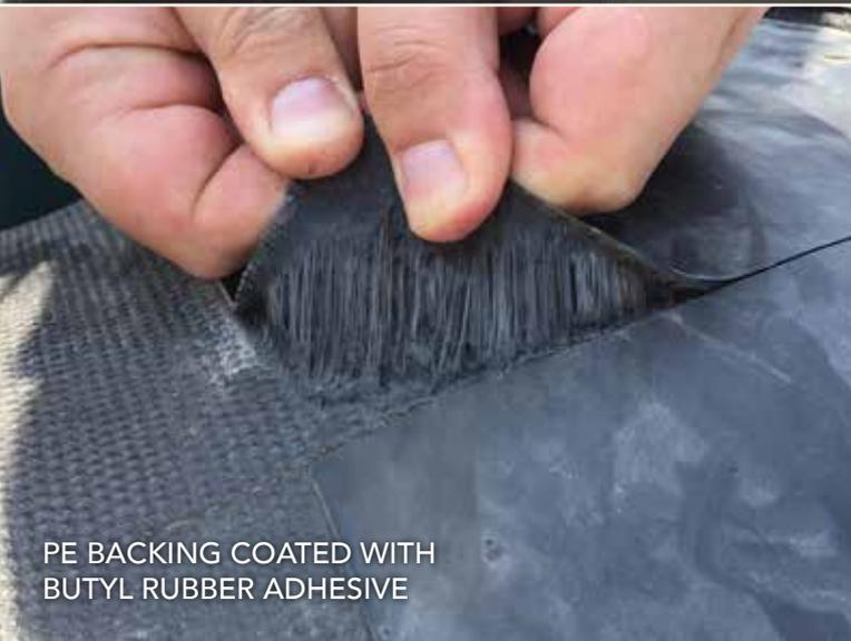
PE BACKING COATED WITH BUTYL RUBBER ADHESIVE
