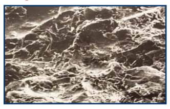
500 x magnification of a steel plate wet-abrasive blasted with HoldTight 102
