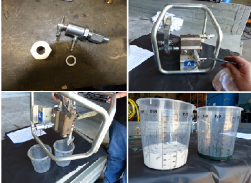
(Top row: Ratio test kit fitted to remote mix manifold Bottom row: 3 Part A to 1 Part B, by volume)
