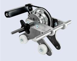
Hand wrapping machines are built to assist in the application of both inner and outer butyl tapes. Using the wrapping machine allows the applicator to set the correct tension and correct tape overlap required.
