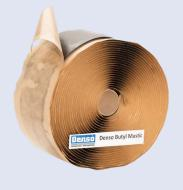
A combination filler and tape wrapping to fill holes and cracks in factory coated pipes, contouring weld beads and cut backs prior to wrapping welded joints, contouring seams on spiral and seam welded pipe, filling/wrapping of bolted connections in junction boxes and sealing exposed electrical cable ends.
