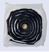
Denso JGR Mastic is a round, non-hardening, tacky, butyl based sealant strip. It is a permanently non-hardening butyl mastic, which can be moulded by hand and is ideal for the sealing of manholes and segmented concrete joints.
