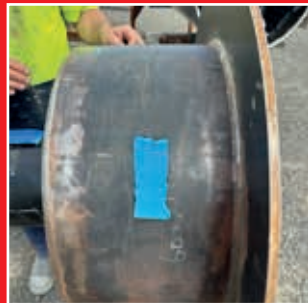
2. Field Viscowrap ST peel test.
